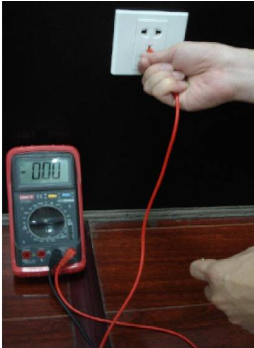
Appendix Figure 7-5 Check earth cable connection
